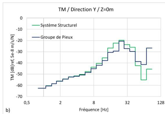
Figure 3 : a) Transfer mobility for the "Free-Field" model at different depths b) Transfer mobility calculated at the surface for the "Group of piles" and "Structural System" models
