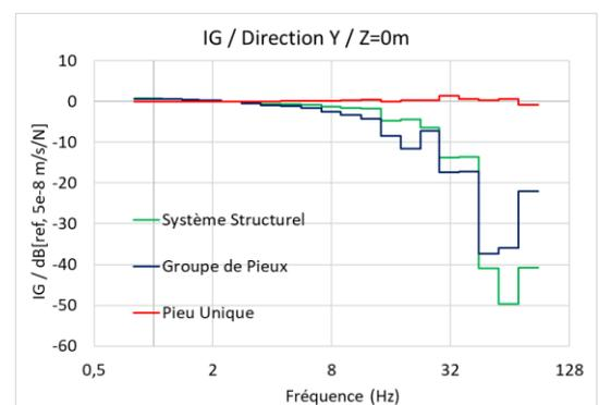
Figure 4 : Insertion gain in the Y direction for the 3 models
