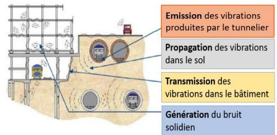
Figure 1 : General Method for Evaluating Vibrations Transmitted through the Soil (ISO 14837-1:2005)
