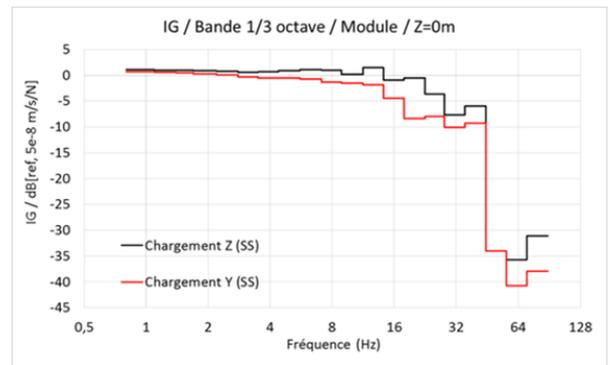
Figure 5 : Insertion gain for normal and tangential loading according to the "Structural System" model
